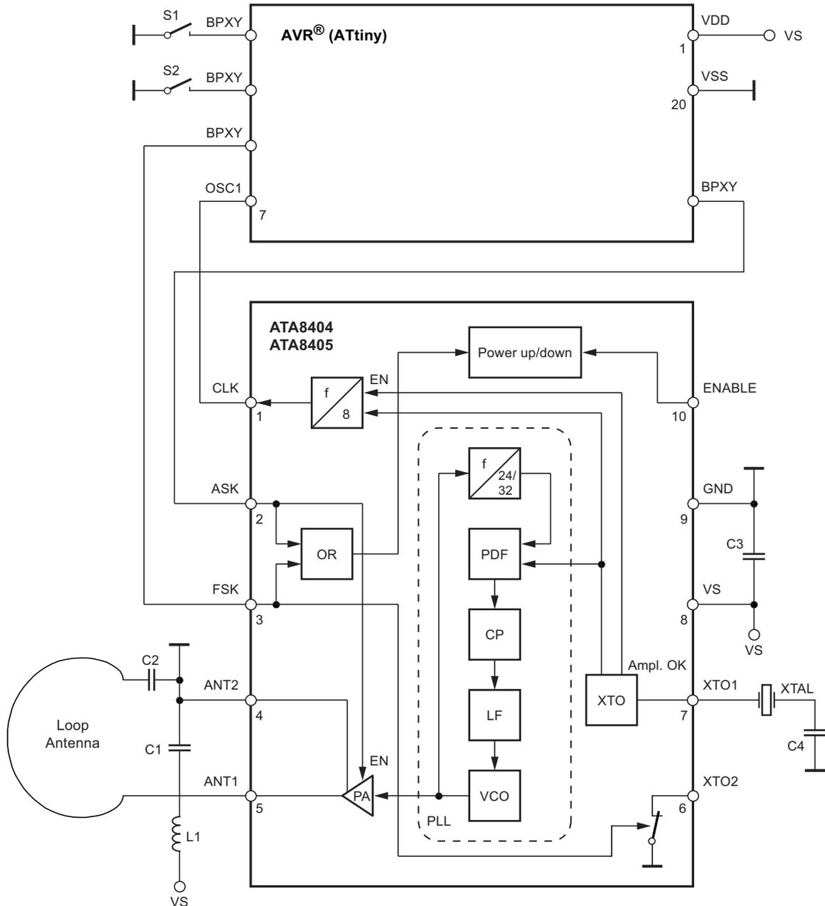
Figure 4-8. FSK Application Circuit
